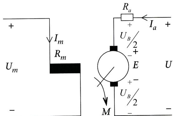
$$\underline{\text{FALL I:}} \quad U = 190 \text{ V} \quad n_I = 820 \text{ RPM} \quad J_{aI} = 25 \text{ A}$$
